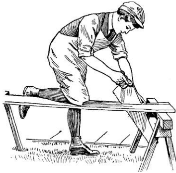
Fig. 15 —Correct Angle of Saw
