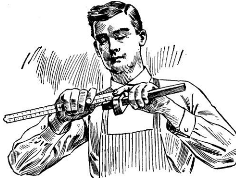
Fig. 36—Holding and Setting Marking Gauge
