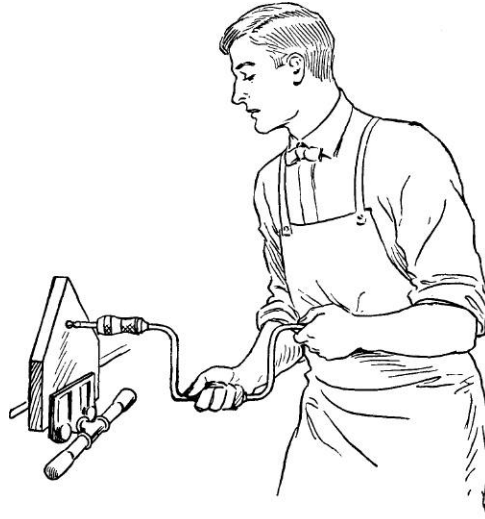
Fig. 62 —Boring a Hole
