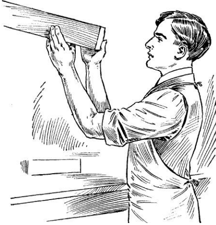
Fig-. 43 — Testing for Straightness
