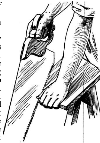
Fig. 14—Guiding the Saw with Left Thumb
