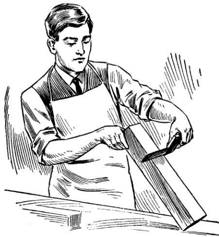
Fig. 47—Testing Across the Grain
