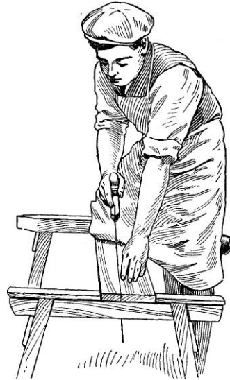
Fig. 16 —Saw, "Wrist and Elbow in One Plane"
