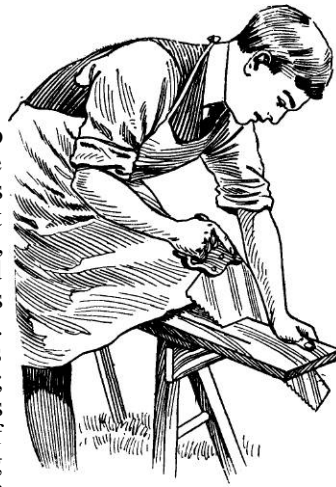
Fig. 17—Holding Overhanging Piece
