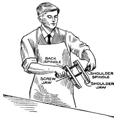
Fig. 85—Rotating a Clamp
